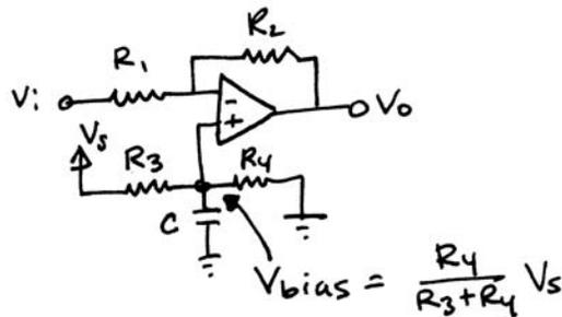
$$G_{AIN} = -\frac{R_2}{R_1} = -G \rightarrow \boxed{G = \frac{R_2}{R_1}}$$
