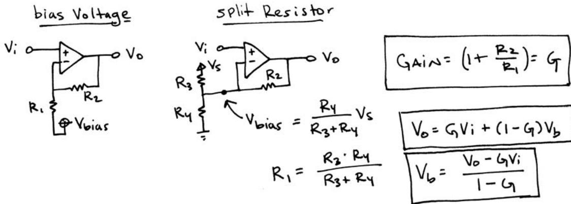
$$\frac{V_i - V_b}{R_1} = \frac{V_o - V_i}{R_2} \rightarrow V_o = \frac{R_2}{R_1}(V_i - V_b) + V_i$$
