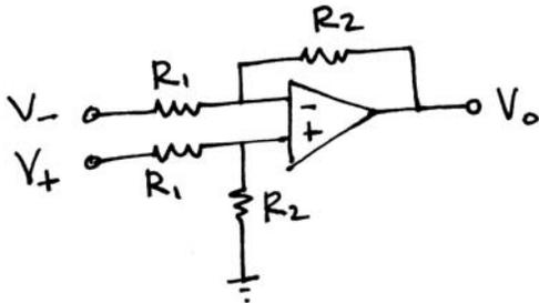
$$\text{GAIN} = \frac{R_2}{R_1} (V_+ - V_-)$$
