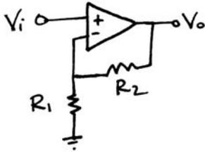
$$\text{GAIN} = 1 + \frac{R_2}{R_1}$$
