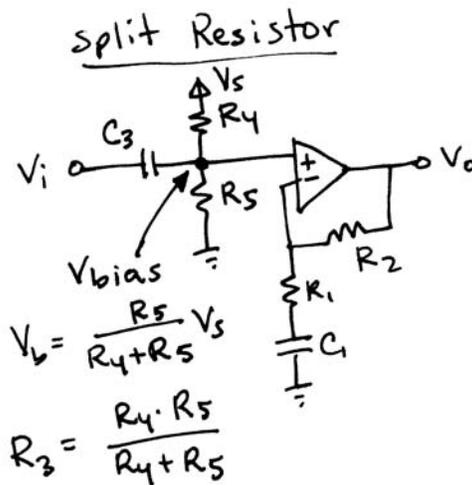
$$\text{GAIN} = \left(1 + \frac{R_2}{R_1}\right) = G$$
